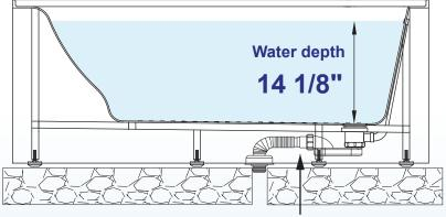
Anti- leak drain and pipe
