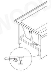
Lock the adjustment by tighten the hexagon nut.
