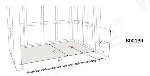
Cut subfloor to accommodate plumbing in compliance with local plumbing and building code. Verify your bathtub for final dimensions.
