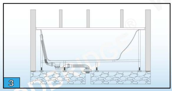
The bathtub can be leveled by adjusting the feet. Check your adjustment with a level
