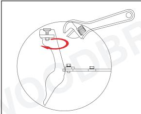
4. Fit the foot to the metal bar and tub , locking washer and bolt . then adjust the stopper foot that touch the ground
