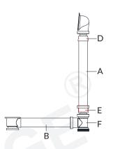
9. Measure the distance between two measure and mark each pipe so that the end of the pipe reaches a little over halfway into the overflow tee. Attention: only pipe "A" need to be cut & fit.
