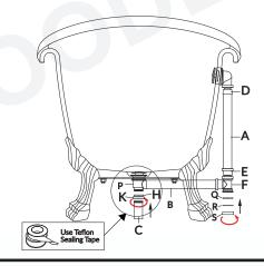
17. Attached the drain tube and flange to the waste and overflow tee with the sealing washer and slip nut.
