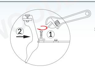
3. Thread a washer and nut onto each stub. Don't fully tighten the nuts: The bar needs to be able to slide back and forth to allow adjustment until the foot is attached.
