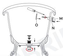
6. Installation of Overflow, Installation of toe shoe.
