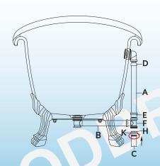
14. Only install " C" as drain is at location shown and attached the drain tube " C" and flange.
