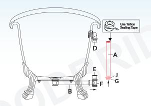
11. Connect Overflow "A" with "D" and "E". Please apply Teflon Sealing tape. Please connect "D" before "E".
