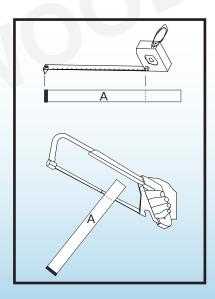
10. Trim the pipes at the marked locations with a hacksaw. Make sure that the blade is suitable for cutting metal.
