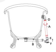
12. The overflow tee will be attached at the points where the drain pipes intersect.
