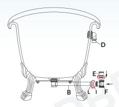
8. Installation of "E" connector with "F". Please refer back to Diagram I for details.
