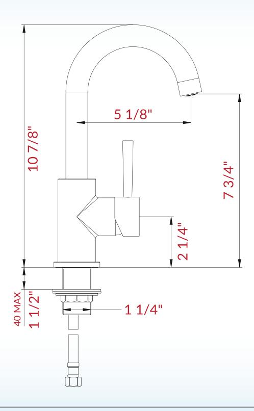
**ATTENTION!** Dimensions may vary by up to 3/8". It is highly recommended to pull all dimensions of actual model for installation and measuring purposes.
