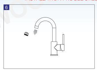
After installation is complete, remove aerator and rotate handle to the closed position. Turn on the water supply valves, and check all connections for a leak. Turn on your faucet and allow both hot and cold water to run at least one minute each. Replace Aerator.
