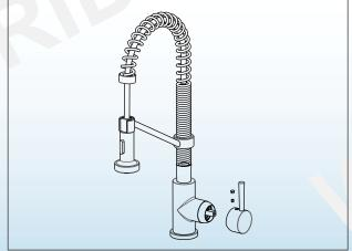
Turn off water and relieve pressure! Detach handle button using a small flathead screwdriver, unscrew set screw using Allen Wrench and take off handle.
