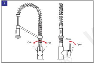
Lift the handle up, the cartridge will be activated allowing water to flow. The water flow will increase by continuing to rotate handle. By rotating the handle to the right, the water temperature will decrease to cold flow only. By rotating Handle to the left, the water temperature will increase to hot only.
