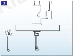
If necessary, tighten screws using a adjustable wrench until the faucet is firmly connected to the sink.
