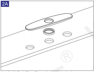
Install with Deck Plate. Place a bead of plumber's putty between faucet and sink. Place Deck Plate over the three holes of sink. From underside sink, tighten Wing nut.
