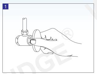
You should clean all the dirts from valve outlets. Turning off the water supply valves. This is usually found near the water meter. If you are replacing an existing faucet, remove the faucet from the sink and clean the sink surface thoroughly.
