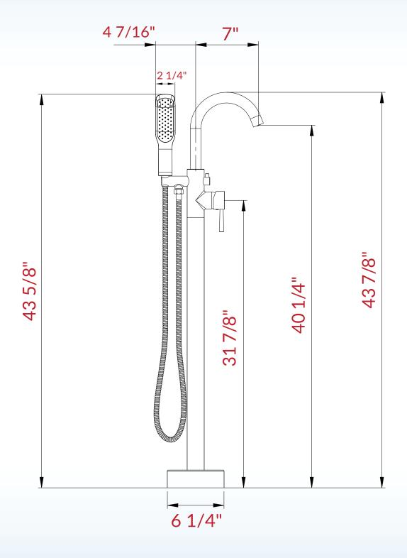
**ATTENTION!** Dimensions may vary by up to 3/8". It is highly recommended to pull all dimensions of actual model for installation and measuring purposes.
