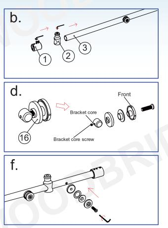
3. Use the Allen Key (19) to loose the screw on the Guide Rail Brackets (1) and Glass Door Stoppers (2). Slide the Glass Door Stopper and then the Guide Rail Bracket to the Guide Rail (3), use the Allen Key to tighten the parts to the guide rail temporarily.
