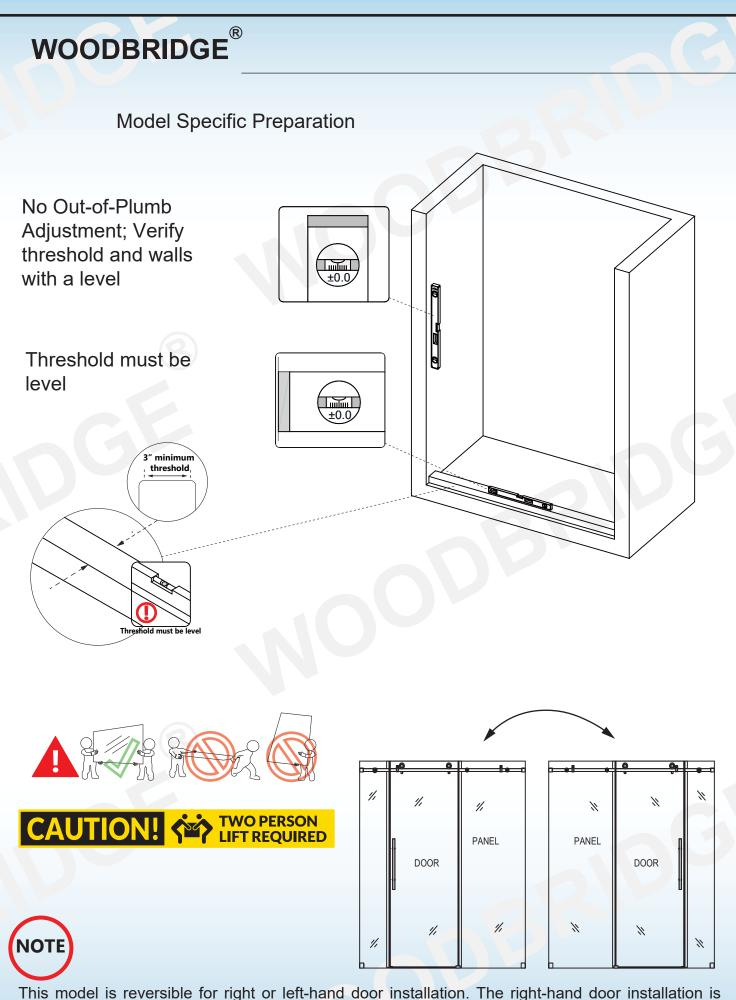
This model is reversible for right or left-hand door installation. The right-hand door installation is shown as an example throughout this manual. For the left-hand door installation, simply begin on the opposite wall and reverse the orientation of the steps shown.
