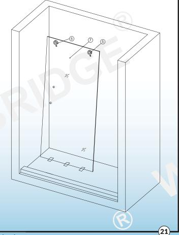
10. Place the Stationary Glass Assembly back into the designated position. Slide the Guide Rail Bracket (1) to the two end sides of the Upper Guide Rail(3). Tighten the set screws on the Guide rail bracket (1) with Allen Key (19) to secure the guide rail to the wall. Install the Bottom Clamp (13) back to the Stationary Glass(14).
