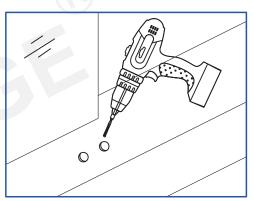
15. Place the Bottom Guide (12) to the bottom edge of the Stationary Glass(14), mark down the predrilled position of the Bottom Guide.
