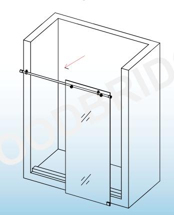
7.Slide the Guide Rail Bracket (1) against the wall, outline the Guide Rail Brackets position on the wall. Set the Stationary Glass (14) aside. Remove the Wall Bracket from the Guide Rail Bracket and place them to the outlined positions and mark the drilling holes on the wall. Outline the position of the Bottom Clamp (13) on the base as well. Remove the Clamp from the Stationary Glass and place it back to the outlined positions, now mark the drilling holes on the threshold.
