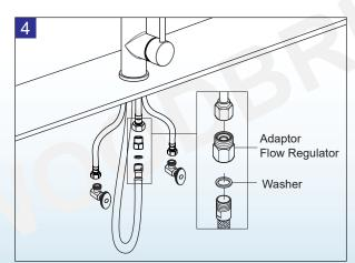
install brass adapter to the hose inlet from below, Connect hot and cold water supply lines to the Water Supply Valves.
