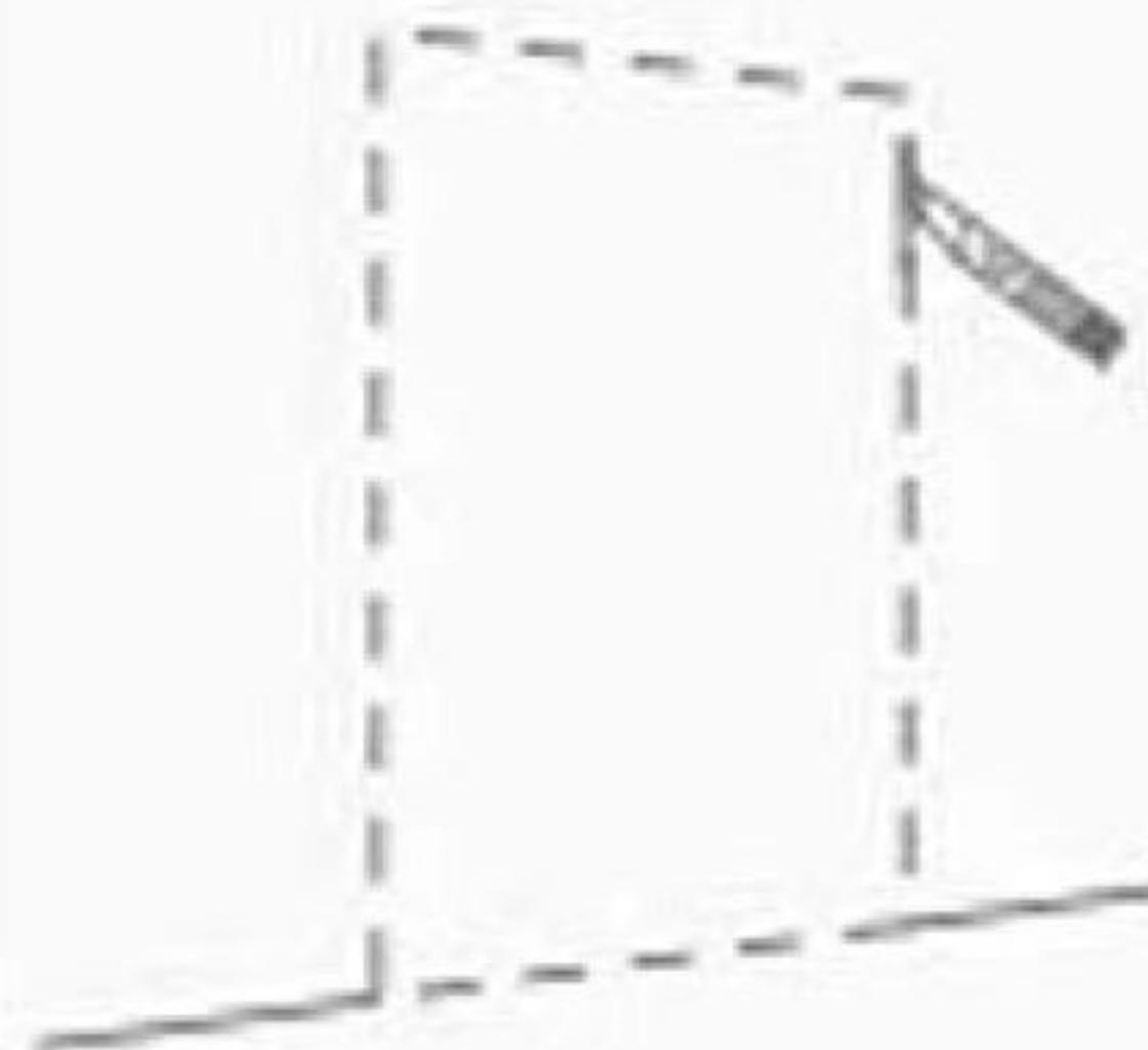
Step1:Track the rough-in size around the entire niche and cut the substrate from the marked traces.
