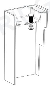
(2) Connect flexi hose drain to the drain assembly as drawing.
