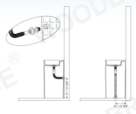
(4) Place the pedestal sink against the wall, put a level on top of the sink and make sure it is level and stable, any minor adjustment if necessary. Apply a beard of silicone caulking around the edge of the pedestal sink and let it dry.
