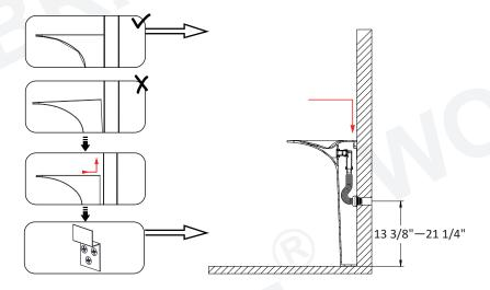
(5) Make sure the sink is flush to the wall, put a level on top of the sink and make sure it is level and stable, any minor adjustment if necessary. Apply a beard of silicone caulking around the edge of the pedestal sink and let it dry.
