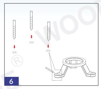
Step 6: Secure the mounting tripod onto the floor using the attached mounting screws.
