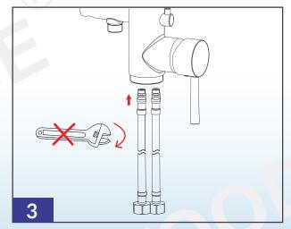
Step 3: Hand tighen the hot and cold flexible water supply line onto faucet body.
