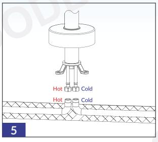
Step 5: Locate the faucet assembly onto the rough valves from floor, and secure the connection of inlet supply lines to the valves. DO NOT reverse the Hot and Cold supply.
