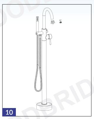
Step 10: Remove the aerator from the spout (if any) and switch the diverter from hand held shower to spout mode and and let both hot and cold water flush for one minute to clear any debris from water lines. Replace aerator and faucet is ready to use.
