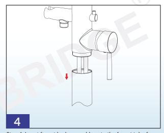
Step 4: Insert faucet body assembly onto the faucet tube from the top and hand tighen it. Make sure the flexible water supply lines go through the tube smoothly.
