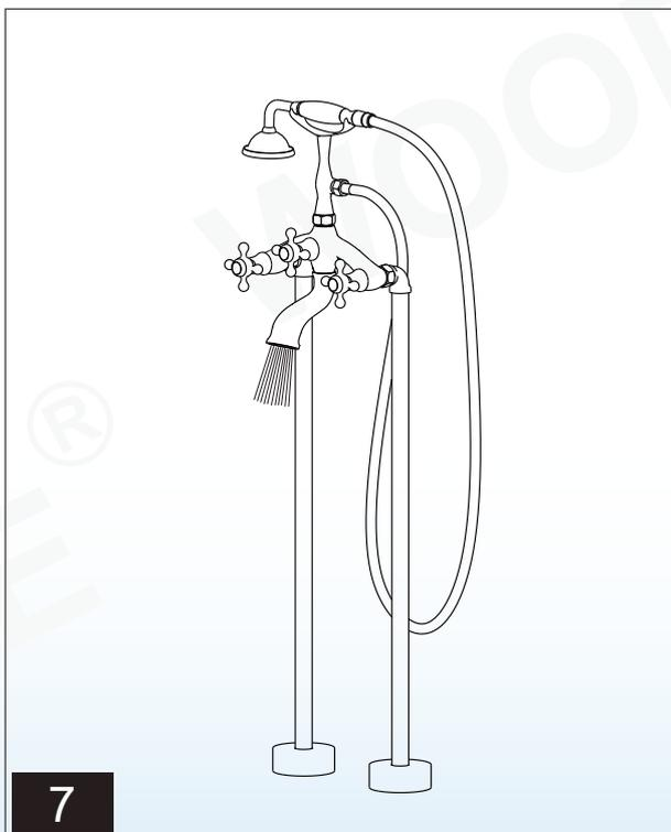
Turn on the both Hot and Cold water valves on the faucet and let the water run for at least one minute to clear any debris from the supply line. Hold hand shower hose and switch the diverter in the middle to hand shower mode and perform the same procedure. Check for any leaks, use wrench to tighten if necessary.
