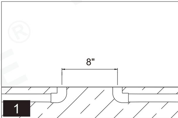
Install water inlet pipe under the floor and make sure the rough in is 8-inches between Hot and Cold water line.
