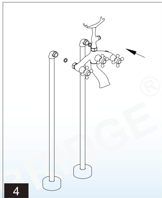
Place rubber washers onto faucet body joint and secure faucet body to riser, hand tighten the Joint, use wrench for adjustment.
