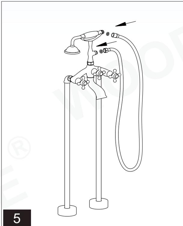
Place rubber washers onto both end of the handshower hose and connect one end of the hose to cradle and the other end to the handshower.
