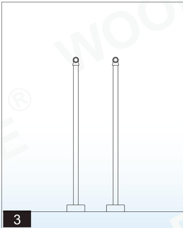
Gently slide down the escutcheon and flushed with the floor.
