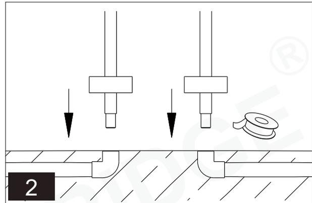
Insert risers through escutcheon , apply 3 to 4 layers of teplon tape on all the threads, connect risers to water inlet from the floor, then align risers and union adapters are facing the tub.
