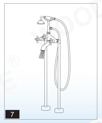
Turn on the both Hot and Cold water valves on the faucet and let the water run for at least one minute to clear any debris from the supply line. Hold hand shower hose and switch the diverter in the middle to hand shower mode and perform the same procedure. Check for any leaks, use wrench to tighen if necessary.
