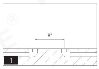
Install water inlet pipe under the floor and make sure the rough in is 8-inches between Hot and Cold water line.
