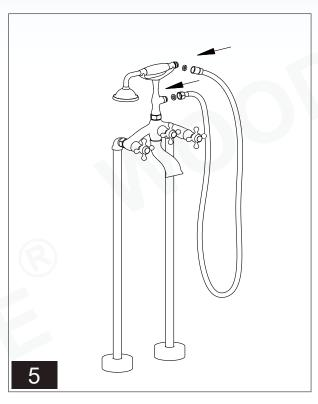
Place rubber washers onto both end of the handshower hose and connect one end of the hose to cradle and the other end to the handshower.
