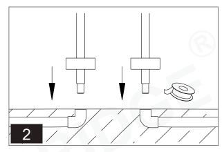
Insert risers through escutcheon, apply 3 to 4 layers of teplon tape on all the threads, connect risers to water inlet from the floor, then align risers and union adapters are facing the tub.
