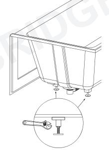
Lock the adjustment by tighten the hexagon nut.
