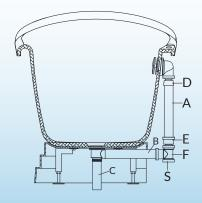
13. When your tub is in place and all connections have been made. Fill the tub with water to check for any leaks from the connections. Verify that the drain and overflow are working properly.
