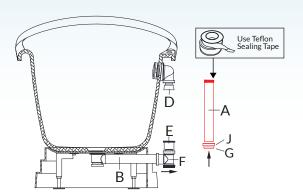
6. Connect Overflow "A" with "D" and "E".Please apply Teflon Sealing tape. Please connect "D" before "E".
