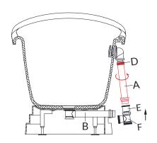
7. The overflow tee will be attached at the points where the drain pipes intersect.
