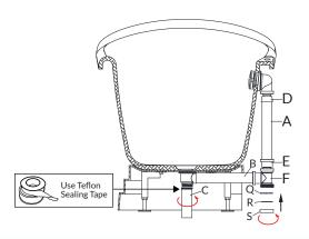
12. Attached the drain tube and flange to the waste and overflow tee with the sealing washer and slip nut.
