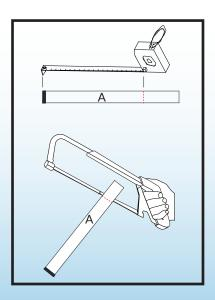
5. Trim the pipes at the marked locations with a hacksaw. Make sure that the blade is suitable for cutting metal.
