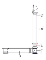
4. Measure the distance between two measure and mark each pipe so that the end of the pipe reaches a little over halfway into the overflow tee. Attention: only pipe "A" need to be cut & fit.
