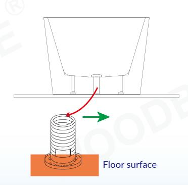
5. Clean the surrounding of the drain pipe with cloth in preparation of setting the drain, the area should be dry and free of any debris. Apply a bead of clear silicon or plumber putty around the drain body and pass it through the drain hole, also apply plumber putty to the washer and slide it over the bottom of the drain body.
