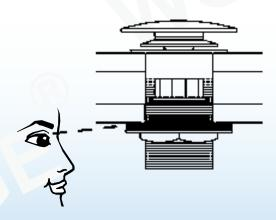
8. Fill the tub with water to the overflow and then drain the tub while inspecting the waste and overflow connection below the floor for any leaks. Access from below will be necessary for this step.
