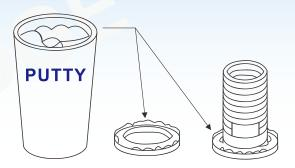
6. Install 1  $\frac{1}{2}$ " rubber slip gasket over the drain waste vent.
