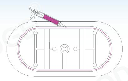
6. Apply a generous bead of adhesive or waterproof silicone to the bottom of the tub and a bead of tub and tile caulk around the edge of the tub
