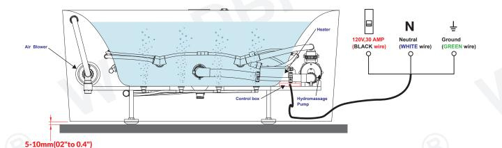
Must hire a licensed electrician to install a dedicated 120V, 30 Amp circuit breaker for the BJ-series-hardwired 3-in-1whirlpool tubs. The electrician also needs to verify the connected electrical wiring can handle a 30 Amp current.
