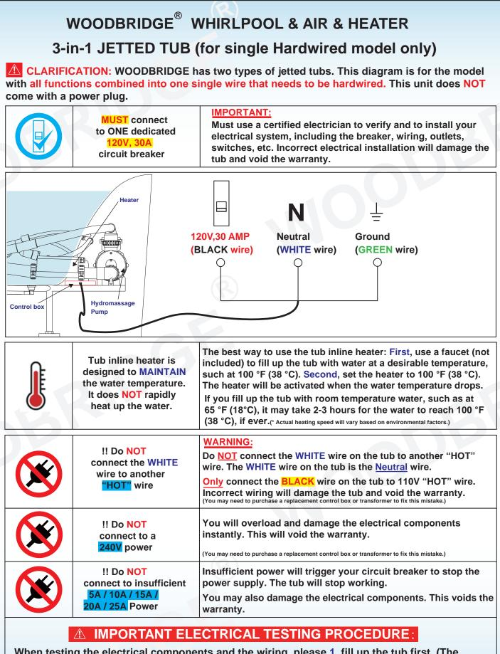
When testing the electrical components and the wiring, please 1. fill up the tub first. (The whirlpool jet cannot to be turned on unless the tub is filled up.) 2.please turn on the whirlpool jet, air bubble blower, and set the heater to 40°C <u>AT THE SAME TIME</u>. 3.Please let it run for 15 minutes. (\* If the water is already hotter than 40°C, you will need to set the inline heater at a higher temperature.)
