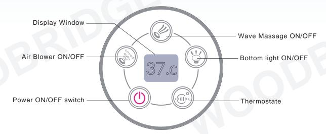
(1) Press the Power switch (b), to turn on the power.
