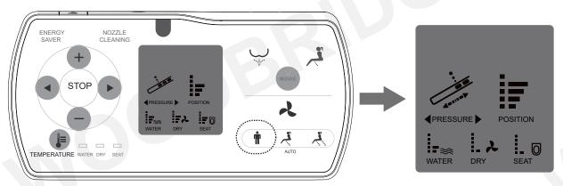
For example, the nozzle position is on level 2, and massage function is open; the water pressure is on level 4; water temperature is on level 2, while dry temperature and seat temperature are on level 1.
