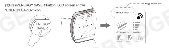
(2)Press"ENERGY SAVER"button again, LCD screen shows figure "6", and the "ENERGY SAVER"icon disappear after 3 seconds, the setting succeeds. The toilet enters the energy saver mode from 9:00 to 15:00 every day. During this period, power light is off, and the energy saver light is on. It goes back to normal operation mode after energy saver time.
