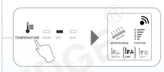
Press "TEMPERATURE" button twice, "DRY" light is on, and icon on the screen lights on, then adjust wind temperature by "+", "-" button. It is regarded as operation completed if there is no operation in 5 seconds, and then "DRY" light is off, icon disappears. Long press "-" button until the "DRY" icon disappears to close the "DRY" function.
