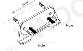
(3)Install battery and place remote control to the hanger.
