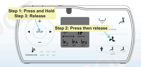
Please note night light feature is default at the off status because the room must be completely dark for the light to turn on. Repeat the process and the night light will switch to intelligent status. Repeat above process constantly, the night light will switch between off status and intelligent status.
