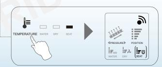
Press "TEMPERATURE" button three times, "SEAT" light is on, and [in graphic icon on the screen lights on, then adjust seat temperature by "+", "-" button. It is regarded as operation completed if there is no operation in 5 seconds, and then "SEAT" light is off, [icon disappears. Long press "-" button until the "SEAT" icon disappears to close the "SEAT" function.
