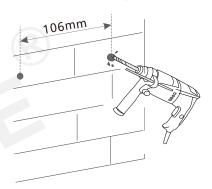
(2)Insert expansion tube into the hole on the wall, install the hanger to the wall with a screw, and paste the double faced adhesive tape on hanger to the wall, tighten
