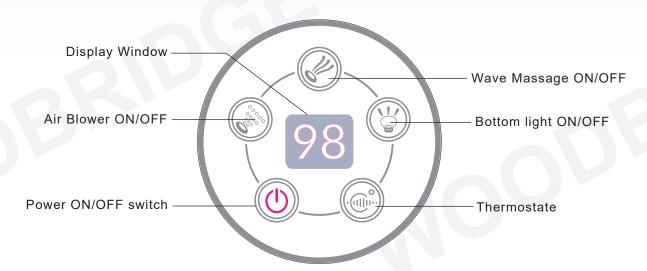
When the power is ON, the number 188 will display on the LED control panel and will disappear after 3 seconds. The power is on and ready to work.
