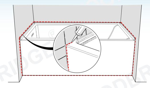
Reference for Correct Tile Flange Installation. Use drawing below as a reference guide for rough-in measurements.
